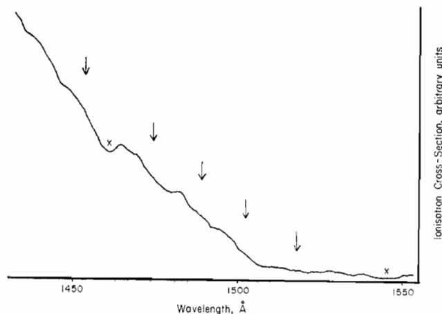
Figure 2.—Relative ionization cross-section plot against wavelength for tungsten hexacarbonyl in the region of the onset. The dips in the curve, marked X, are due to the presence of emission lines in the continuum light source used. The arrows indicate the position of inflections averaged over several runs.
